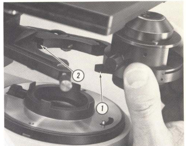
FIG. 12-4 - INSTALLING CONDENSER INTO SUBSTAGE
