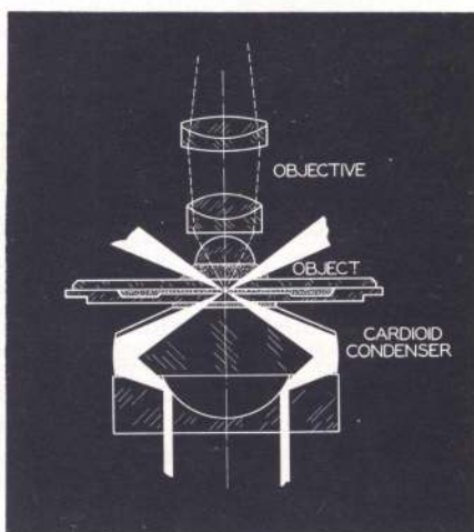
Figure 19—Two types of Darkfield Condensers. Each delivers a hollow intense cone of light, of greater N.A. than the objective N.A., hence objects are seen only by virtue of the light which they scatter.
