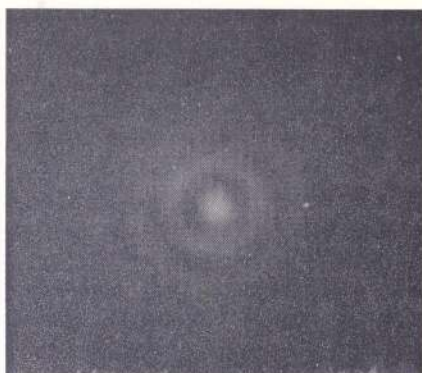
Figure 4—The appearance of the Airy disc when spherical aberration is present. Photomicrograph taken with a 4mm, 0.65 N.A. objective, purposely spaced incorrectly to show the effect of lens spacing on spherical aberration. Compare with Figure 3.
