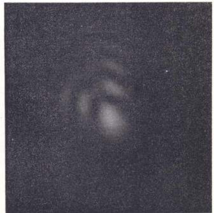
Figure 6—The appearance of a point object due to the presence of coma. Compare with Figure 3.
