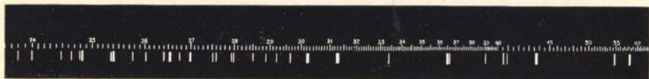
Fig. 7. Spectrum of quartz mercury arc lamp. Made with Bausch & Lomb medium quartz spectrograph. Slit with 5 microns—Aperture F:11.0. Shows the strong triplet at 365 m\mu and only relatively weak lines at 390, 404 and 407. Lines 302 and 312 in the spectrogram are practically cut out by the UV filter. 334 line is partially passed by this filter.
