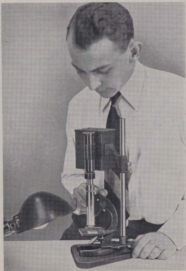
Focusing with the focusing tube when roll film is used
