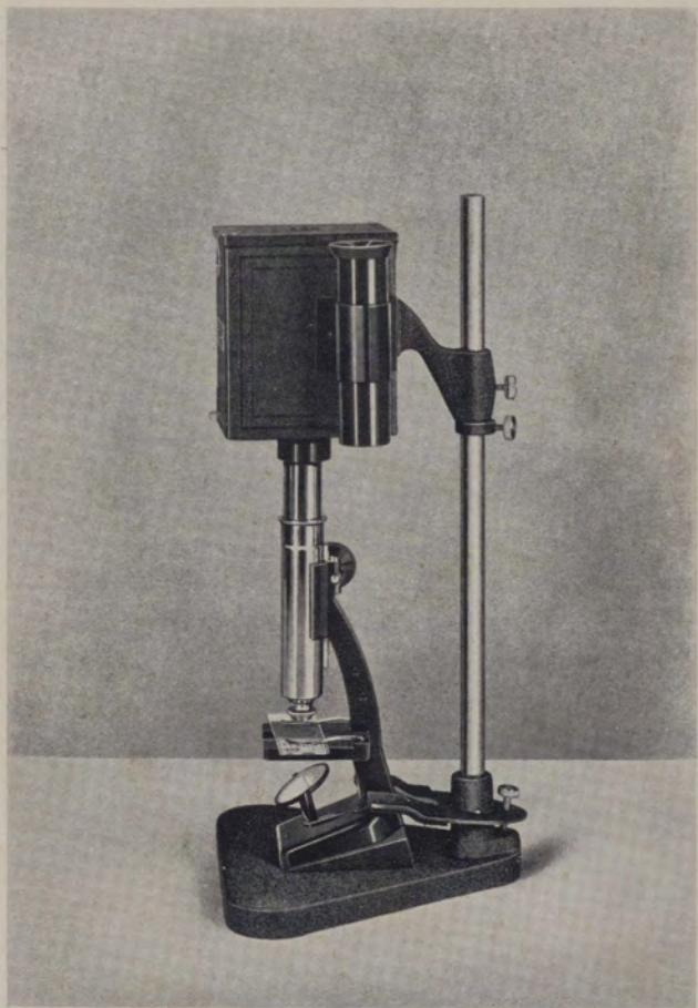
The Photomicrographic Outfit ready for use with Bausch & Lomb's New Gem Microscope. Note the wooden wedge under the base used to bring the body tube to the vertical
