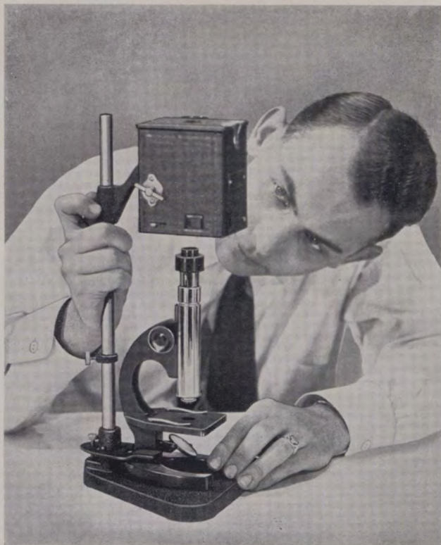
Bringing the microscope into position before clamping to base
