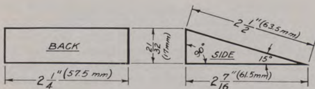
Dimensions of Wooden Wedge Used Under the Base of the Gem Microscope
